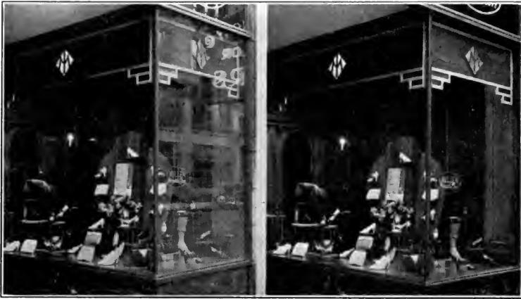
FIG. 5. Shoe store window photographed in daylight with and without the Pola-screen over the lens, to subdue oblique reflections. The Pola-screen is not effective in photographing a window straight on.
